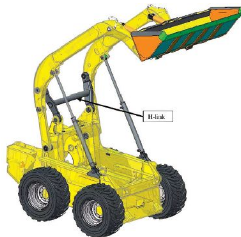
CAD model of vertical lift loader assembly on chassis.
